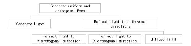
Using Function Tree, it is revealed the functions of 3 films are lower level functions of one functional requirements. Reflect Light to the Screen. Because the thickness of reflector is very thin, the light can't be reflected to the orthogonal direction. Therefore they add lower level functions as refracting light (X-Y direction) and diffuse light.
