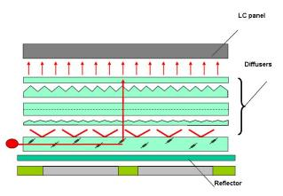
It was because they focused on existing functions of films (1 Diffuser and 2 Prism Film). Firstly, They merged films into one or merged it with other components in the system. But the suggested ideas were too hard to manufacture.
