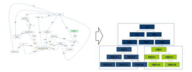
Function Tree is developed for describing functional structure to design future system. It starts from conventional Function Analysis and extract functions from it. It is turned to Functional Requirement and grouped as Function Module. After that it forms a hierarchical structure of sets of Functional Requirements. Function Tree could overview a system more in the philosophical view of designer.
