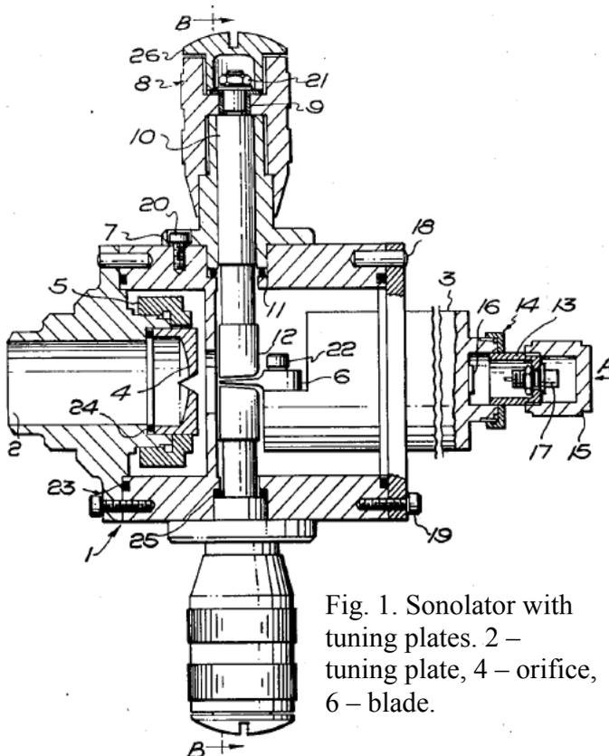
Fig. 1. Sonolator with tuning plates. 2 – tuning plate, 4 – orifice, 6 – blade.
