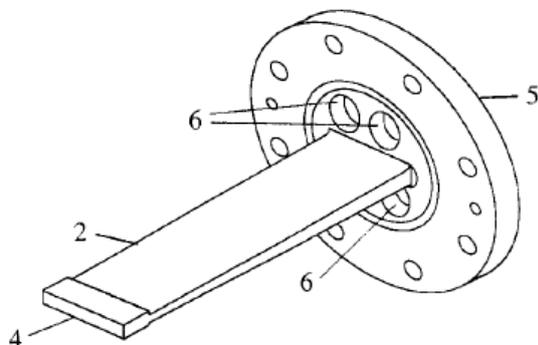
Fig. 2. Weighted blade of the Sonolator. 2 – blade, 4 – weight.
