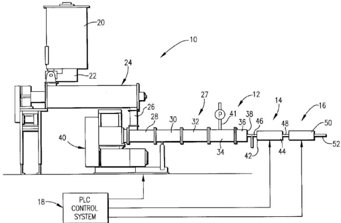
Fig. 3. Homogenizer for Viscous Compositions. 12 – extruder, 14 - Sonolator
