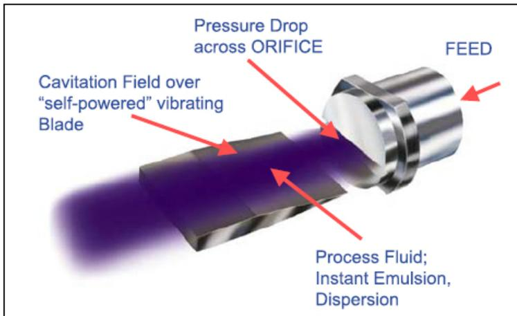
Sonolator is a high-shear mixer, homogenizer and emulsifier which works via ultrasonic cavitation created when a high-velocity liquid jet impacts vibrating blade (see figure at the left). The jet is created by passing a pressurized liquid
